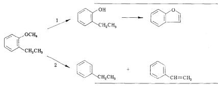
ring (Path 2) which involves a cleavage of the aryl-oxygen bond, leads to ethylbenzene and styrene. In the runs we have made, carbonyl sulfide gave the best selectivity for benzofuran over chromia-alumina, which suggests an important role for the catalyst. However, the thermal reaction is emphatically shown with methane and carbon dioxide over alumina where a catalytic dehydrogenation function is absent.
